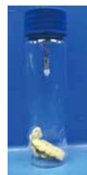
Sampling blue cheese with MonoTrap RGPS TD
